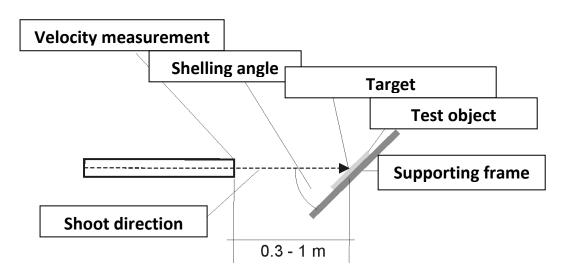
Test velocities are measured by optical lasers. According to the mass of the ice ball and the velocities the impact energy (joule) occurring at the tested object is determined.
